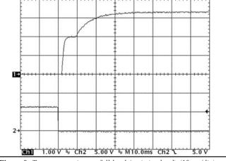
*Figure 9:* Turn-on transient at full load (resistive load) (10 ms/div). Input voltage pre-applied. Top Trace: Vout (1V/div). Bottom Trace: ON/OFF input (5V/div)
