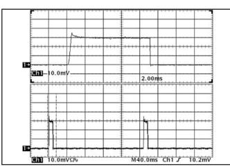
**Figure 18:** Load current (15A/div) as a function of time when the converter attempts to turn on into a 1 m $\Omega$  short circuit. Top trace (2ms/div) is an expansion of the on-time portion of the bottom trace.
