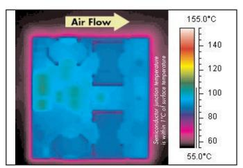
*Figure 6:* Thermal plot of converter at 38 amp load current with 55°C air flowing at the rate of 200 LFM. Air is flowing across the converter from input to output (nominal input voltage).
