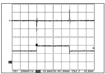
Figure 12: Output voltage response to step-change in load current (50%-75%-50% of Iout(max):  $dI/dt = 5A/\mu s$ ). Load cap:  $480\mu F$ , 15 m $\Omega$  ESR tantalum cap and  $1\mu F$  ceramic cap. Top trace: Vout (200mV/div), Bottom trace: Iout (15A/div).
