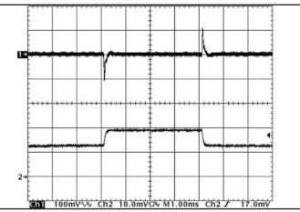
**Figure 11:** Output voltage response to step-change in load current (50%-75%-50% of lout(max);  $dI/dt = 0.1A/\mu s$ ). Load cap:  $15\mu F$ , 450 m $\Omega$  ESR tantalum cap and  $1\mu F$  ceramic cap. Top trace: Vout (100mV/div), Bottom trace: lout (15A/div).
